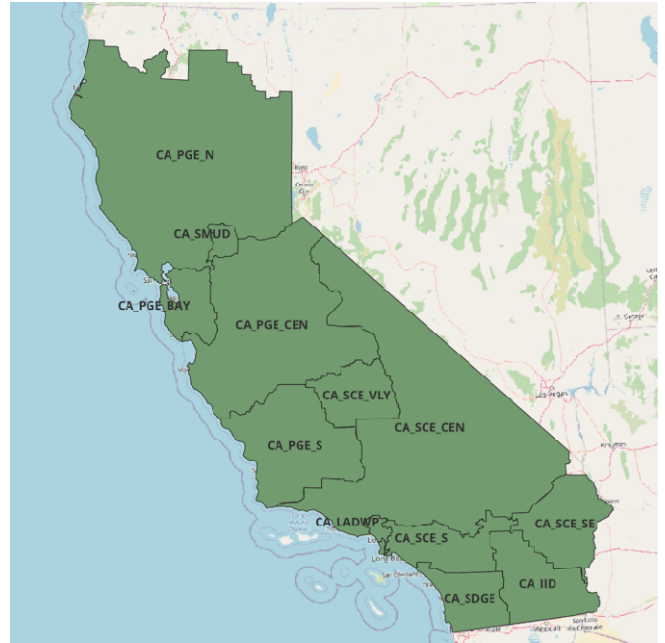
Fig. 1. Grid topology proposed for California. The shape and area of the load zones are similar to those previously developed by the Switch-WECC team.
