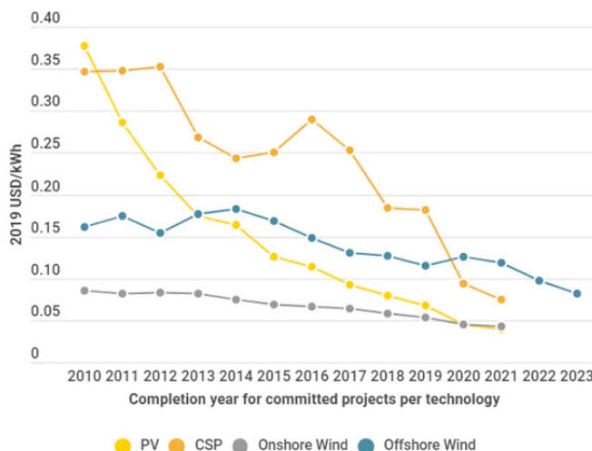
Fig. 2. 7 Cost evolution showing how CSP has recently been catching up with other renewable technologies 20 Deployment of CSP systems may continue to lag those of PV (electricity generation from CSP is less than 10% of that from PV), but CSP’s ability to store heat and generate electricity after the sun sets provides it an advantage in a place like California, where the generation for solar already meets much of the load during the day. Investment in CSP has increased recently. For example, Heliogen just announced $83 million in new funding, providing them with a total of $108 million for their power tower approach. 21 Although Heliogen is focusing on industrial processes rather than electricity generation, such an investment provides a pathway to reduced costs that could also be applied to CSP for electricity generation.
