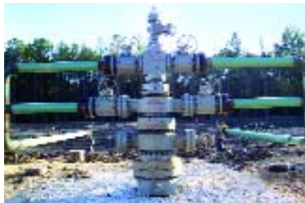
The wellhead situated above the cavern, which is drilled to a depth of 4,600 feet.
