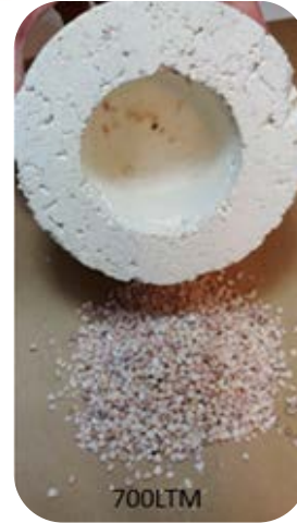
Material thermal stability/compatibility tests at 1200°C
